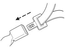
2. To unfasten, press the release button and remove the tongue from the buckle.
